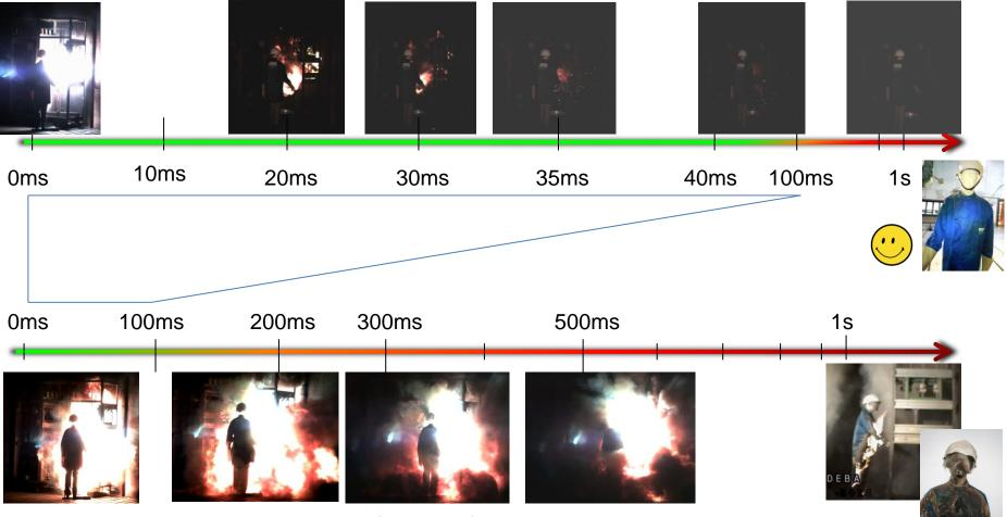
Arc fault inside conventional unit (16kA-1s)
