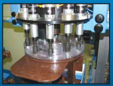
Custom designed machinery control perimeter torque as cover "0" rings are compressed.
